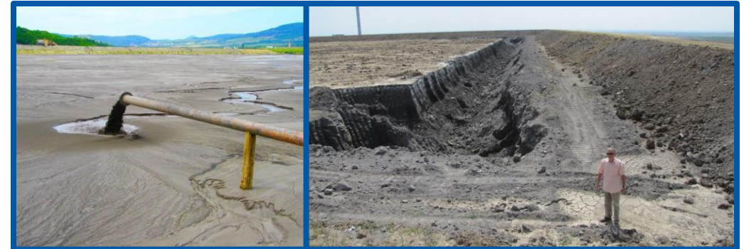
Dense slurry pumped to ash pond and after solidification
