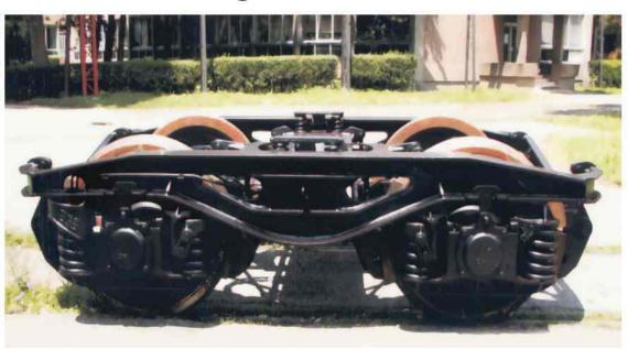
Bogie Y25 Lsd1-K corresponds to TSI, EN, UIC, RIV/AVV, TE regulations. It is designed for maximum running speed of 120 km/h at axle load of 20 t and 100 km/h at axle load of 22,5 t. Wheel sets are with mono-block wheels Ø920 mm, fully according to EN 12060 and EN 13979-1. Brake blocks are made of composite (2 x 250 mm) COSID 810, fulfilling the requests of V-BKS(K) norm for the installation of composite brake blocks. Brake rigging is in accordance with UIC 542 leaflet for "S" regime.
