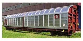
Covered multi-purpose wagon is designed for transport of palletized loads, paper, home appliances, automobile parts, etc. The goods are protected from atmospheric influences. Opening of the lateral sliding doors releases app. 50% of
