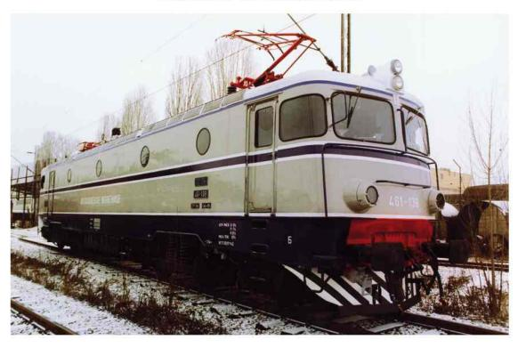
Repairs at Želvoz are mostly performed on six-axle mono-phase diode electro-locomotives for the voltage of 25kV, 50Hz. Beside the repairs, modifications and modernization of control and safety devices are also performed as well as air-conditioning of the driver's cabin.
