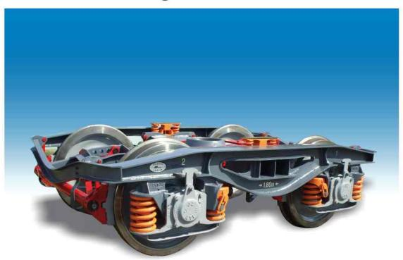
Bogie Y25 Lsd1 corresponds to UIC and RIV/AVV regulations. It is designed for maximum running speed of 120 km/h at axle load of 20 t and 100 km/h at axle load of 22,5 t. Wheel sets are with mono-block wheels Ø920 mm, fully according to EN 12060 and EN 13979-1. Brake rigging is in accordance with UIC 542 leaflet for "S" regime.
