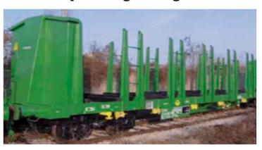
The wagon is produced by reconstruction of Regs type of wagon. The wagon with high sides and fixed pillars is intended for transportation of logs, timbers, pipes and similar. The wagon is equipped with binding hooks and tightening mechanism on lateral sides. The wagon satisfies the requirements of UIC and AVV regulations.
